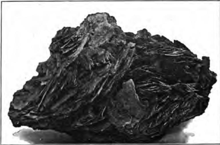
EXHIBIT NO. 1. SCALE BETWEEN SHELL AND TUBES. (C. S. Garrett & Son Co., Buck Run, Pa.)
